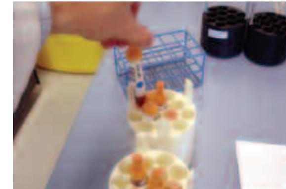
Standardised process: Specimens put directly into centrifuge carriage. This stops double handling. Carriages are loaded directly into centrifuge, eliminating 40 minutes of delays per day.
